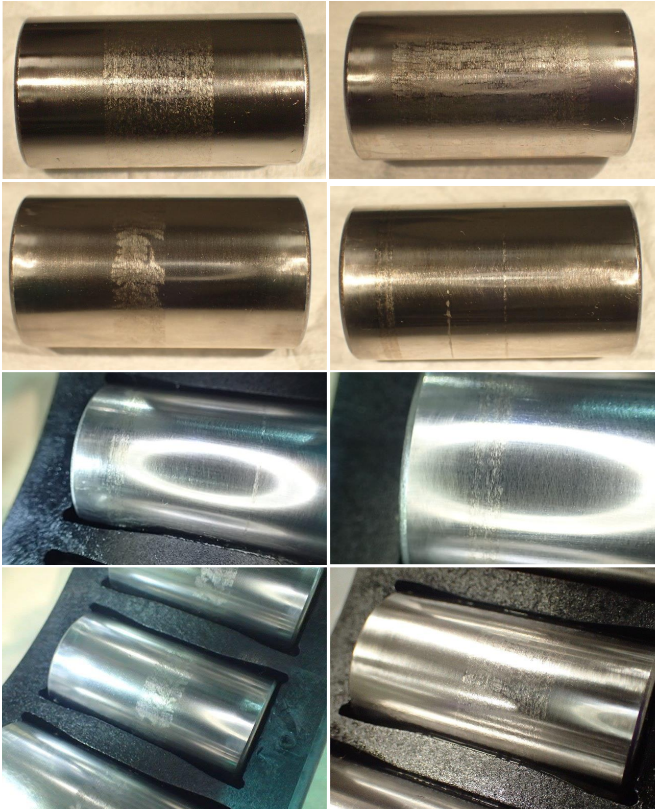
Figure 4: Slippage marks roller
